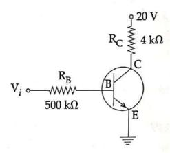
In the circuit shown in the figure, the input voltage  $V_i$  is 20 V,  $V_{BE} = 0$  V and  $V_{CE} = 0$  V, what are the values of  $I_B$ ,  $I_C$  and  $\beta$ ?
